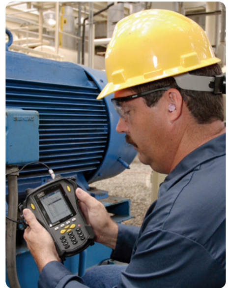
Recording vibration values using an SKF Microlog series data collector
